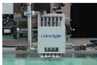
固定头重型冲孔6冲刀 Fixed heavy-duty punching head with 6 punch tool sizes
